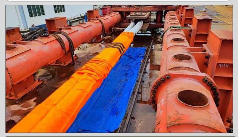
Stybarrow DTM Removal, Australia KimLift® Synthetic Round Slings
